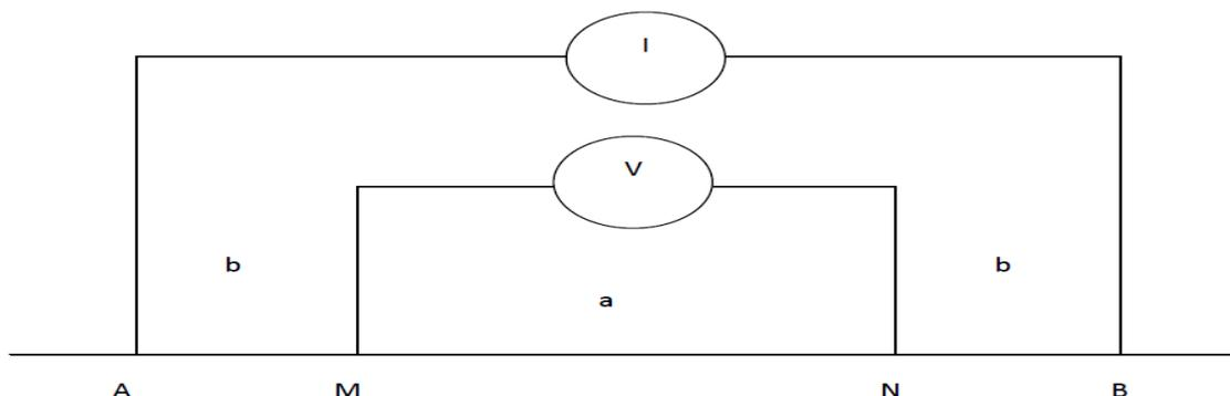
Figure 1: Schlumberger array and apparent resistivity diagram (Keller, 1966)
